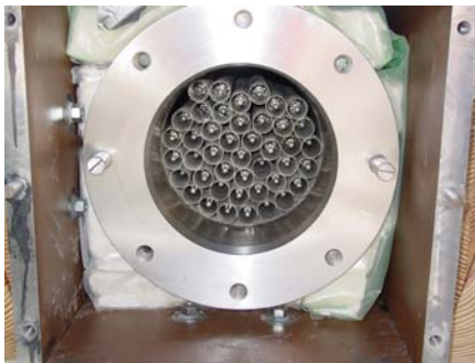
Fuel Rods in WE-1 Container at Penn State
